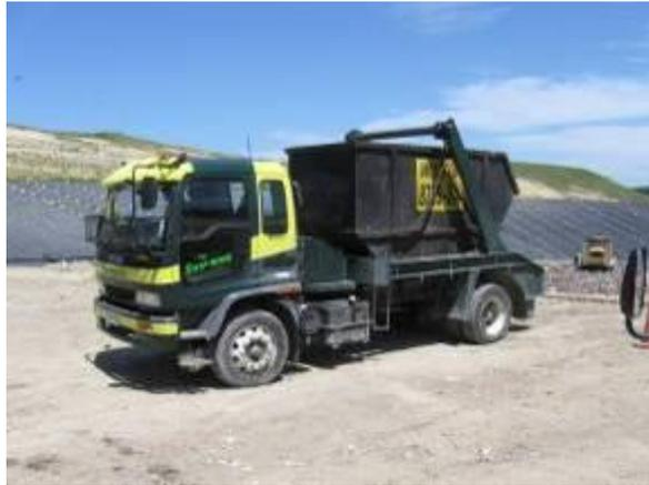
Typical gantry truck loads weigh from 0.5-3 tonnes. As most refuse transported in gantry bins is not compacted, there is often opportunity for manually recovering materials from gantry bins when discharged onto a tipping floor. Gantry bins often contain significant quantities of recoverable materials, such as timber and packaging and reusable items can be recovered intact from residential loads.
