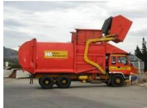
The potential for the recovery of materials from waste transported by front-end loaders is limited. The waste load is compacted by the truck, and the loads tend to be large and heterogeneous. This restricts significantly the potential for manually separating recoverable materials when the load is discharged on a tipping floor. There are usually not significant quantities of easily-separable materials other than cardboard packaging in front-end loader refuse.
