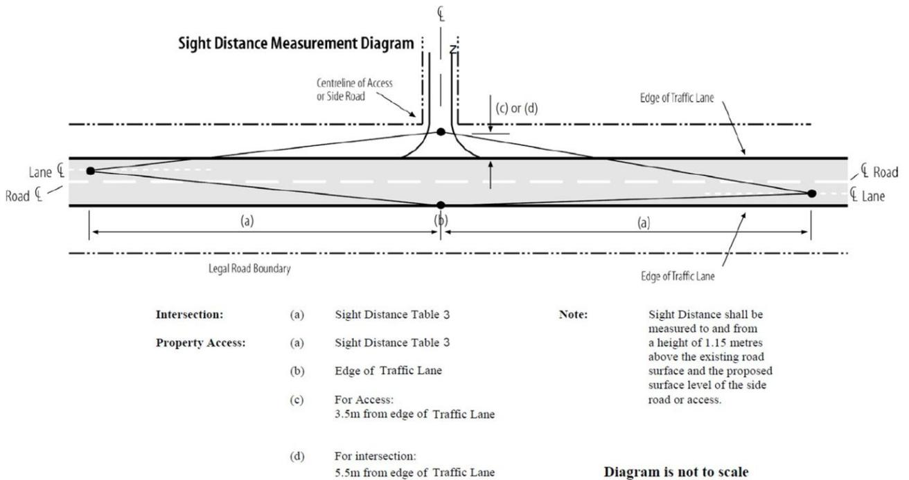
29.14.12 Diagram 12 – Sight Distance Measurement Diagram
