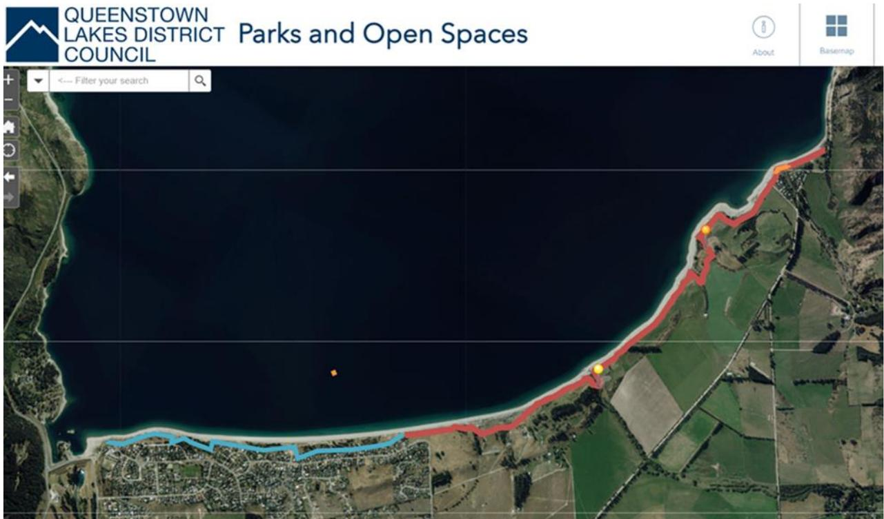
**BLUE:** Heavy maintenance    **RED:** Sub grade reshaping and trail surfacing    **YELLOW:** Bridge
