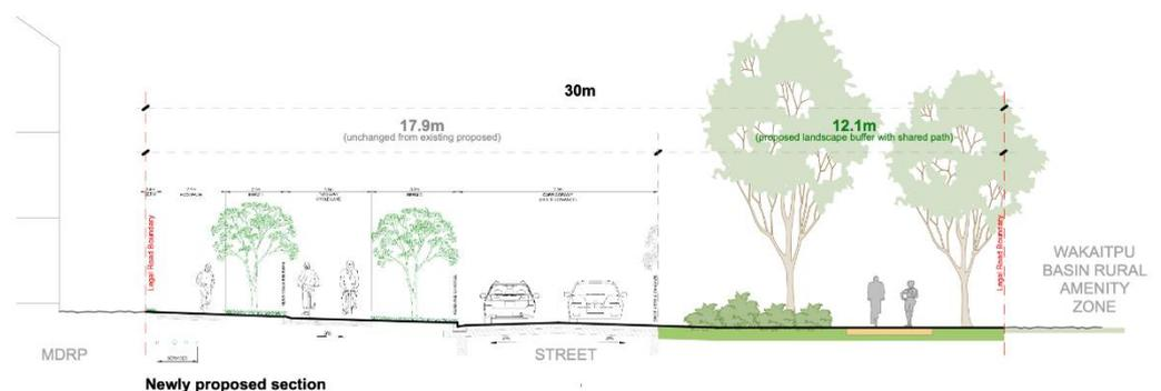
Figure 10: Proposed amendment to Collector Road B cross section
